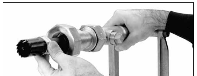
Fig. 3 Attach the Arbor-Driver-Hole Saw assembly to the end of the Boring Bar.
