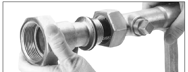
Fig. 2 Select the proper Drilling Machine Adapter and attach it to the Drilling Machine.
