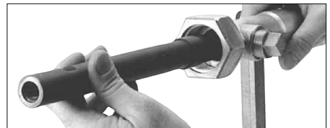
Fig. 1 Insert the Boring Bar into the Drilling Machine.
