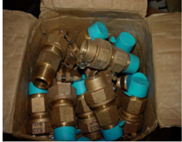
Material thrown into box, improperly packaged
