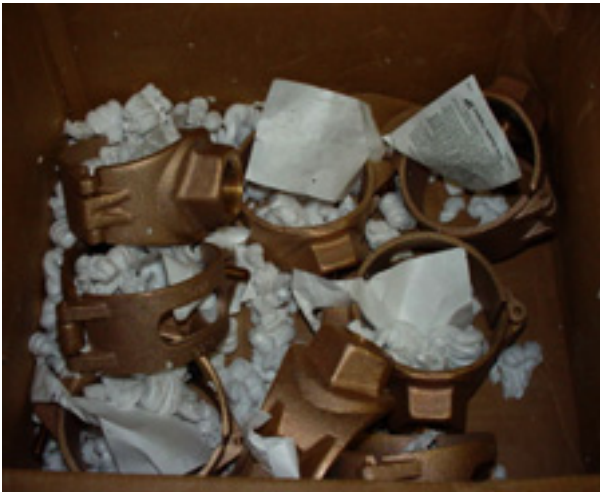
Poor and improper packaging
