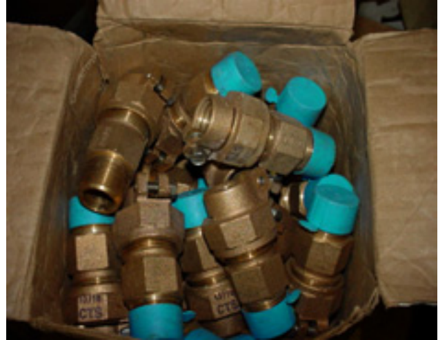
Material thrown into box, improperly packaged
