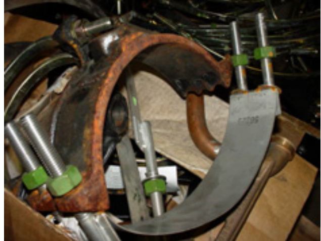
Material rusty, improperly boxed
