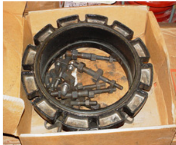
Coupling and hardware rusty
