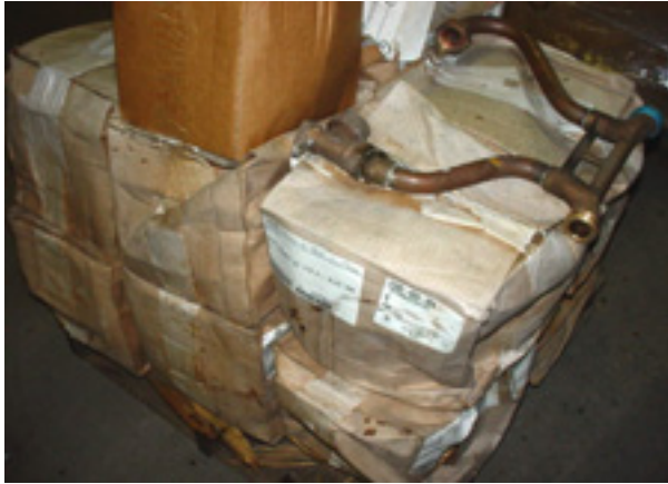
Boxes have been wet now in poor condition, discolored product
