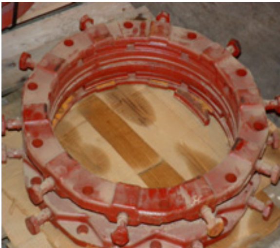
Retainer glands dirty and rusted
