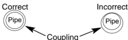
8. Push gaskets (by hand) into center sleeve evenly. Position end rings against the gaskets. Insert and tighten all bolts finger tight. Evenly tighten bolts in an alternating sequence being certain that end rings remain parallel to one another. 1/2" Bolts = 40 - 50 ft. lbs.
