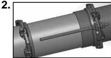
2. Restraint Ring Assembly (1400 with wedges and Auto-Tork Screws): Place the gland with wedges on the spigot end of the pipe with the lip extension toward the face of the pipe bell. Assemble the pipe joint according to pipe manufacturer's recommendations.
