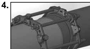
4. Bring all wedges in contact with the pipe surface by turning the Auto-Tork actuating screws in a clockwise direction until the screws are hand tight.
