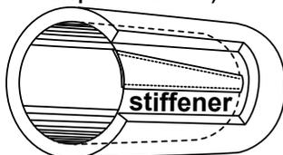
6. Insert the non-dimpled end of the split stiffener into the pipe approximately 2/3 of the insert's length.
