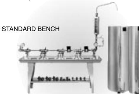
Any test bench that holds both large and small meters is necessarily a compromise. Either the means of clamping domestic sizes (5/8", 3/4" and 1", which in most cases constitute almost 90% of the testing) is
